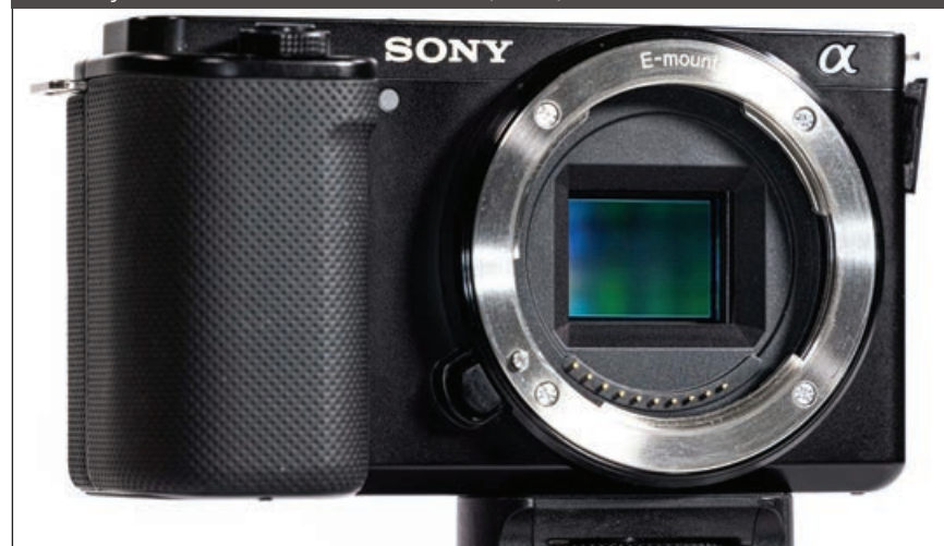
The Sony ZV-E10 houses a 23.5 x 15.6 mm (APS-C) CMOS sensor
