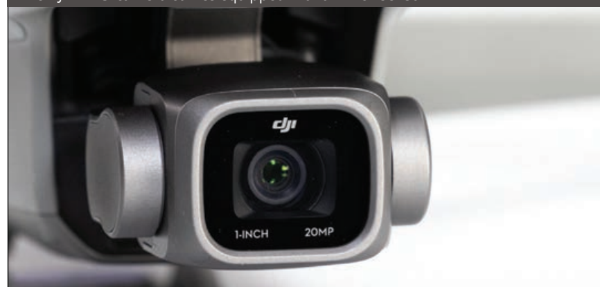
The DJI Air 2S' camera comes equipped with a 1-inch sensor
